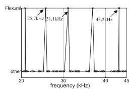
Figure 2: Vibration modes of the 93mmx65mmx0.9mm glass plate. Each cross represents an existing vibration mode.
