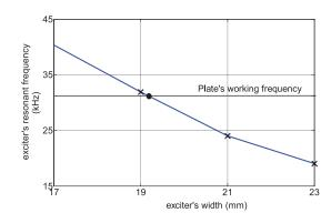
Figure 4: Criterion for exciter's width choice.
