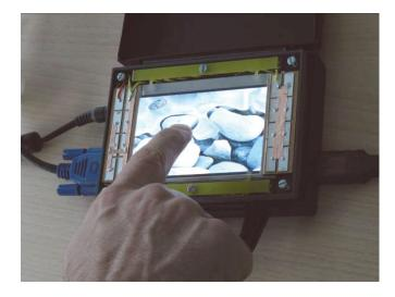
Figure 13: The tactile stimulator In operation.
