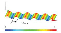
Figure 3: Simulation result of the deflection at 31,2kHz (arbitrary color scale).
