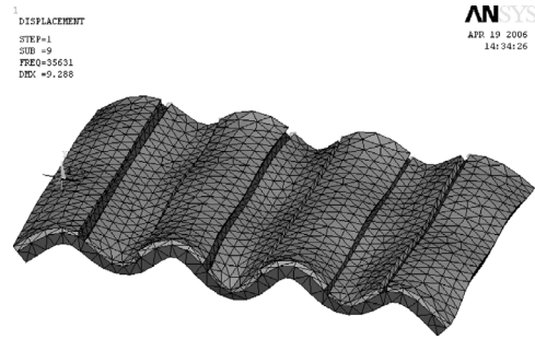
Fig. 11. Result of the modal analysis: deformed shape of the (8;0) mode at f = 35.6 kHz (ANSYS software®).
